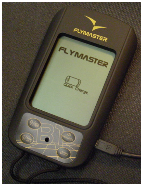
Figure 1 -Battery charge connection
